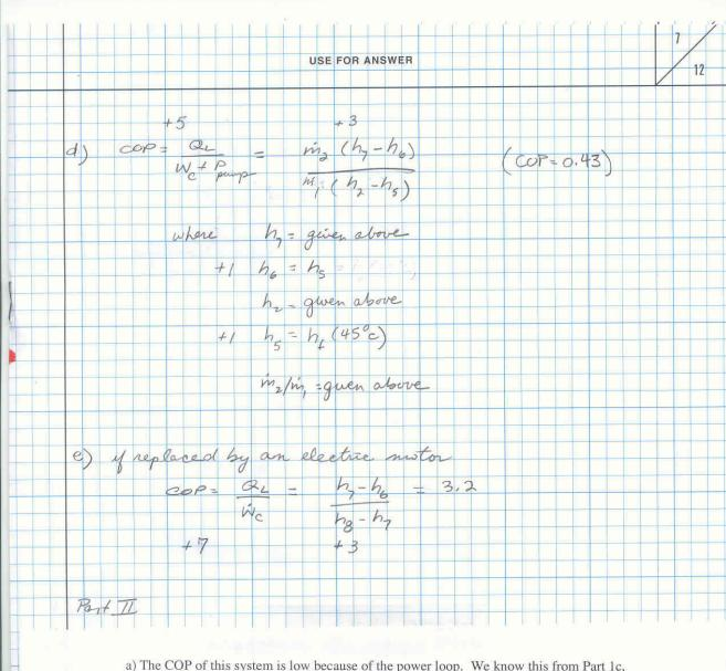
a) The COP of this system is low because of the power loop. We know this from Part 1c, where we found that removing the power loop restored the COP to a typical value of about 3. COPs for refrigerators are always reported without taking into account the efficiency of electric power generation and transmission. If they did, the COP would be less than 1.
